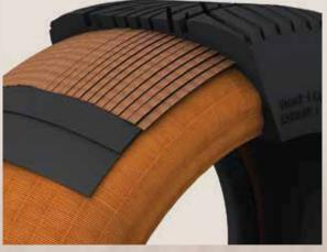
Capmax<sup>TM</sup> has been developed to provide considerable cost reduction for tire makers by eliminating some rubber compound, rubber mixing, calendering, slitting processes, and material scrap from the tire making process. Tailoring the physical properties (Breaking strength, modulus, adhesion and shrink force) according to the customer needs, and Kordsa can make custom design strips with provided structural handling&building integrity.
